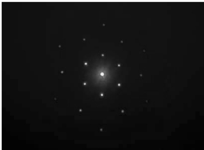
FIGURE 5 Diffraction pattern from a triangular lattice organic photonic crystal.
